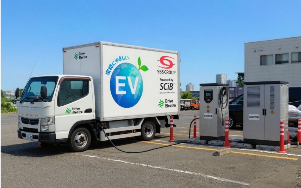
An EV truck retrofitted from diesel
