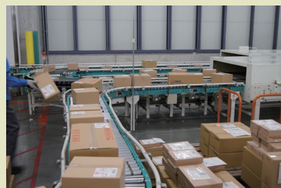
Packed-up products are sorted by automatic sorters by area and shipped.
